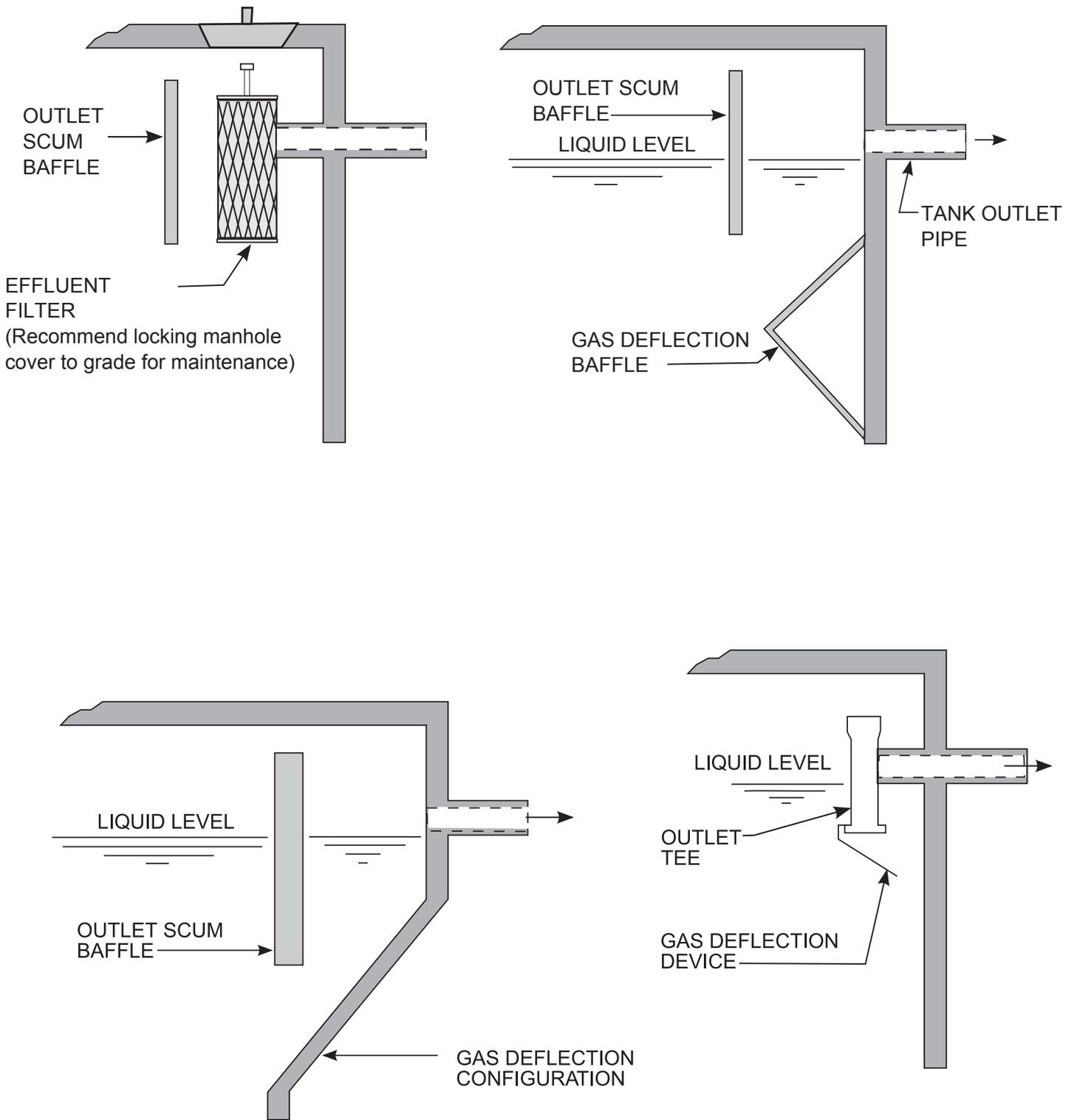
**FIGURE 6: EFFLUENT FILTERS AND SEPTIC TANK OUTLET ENHANCEMENTS**
