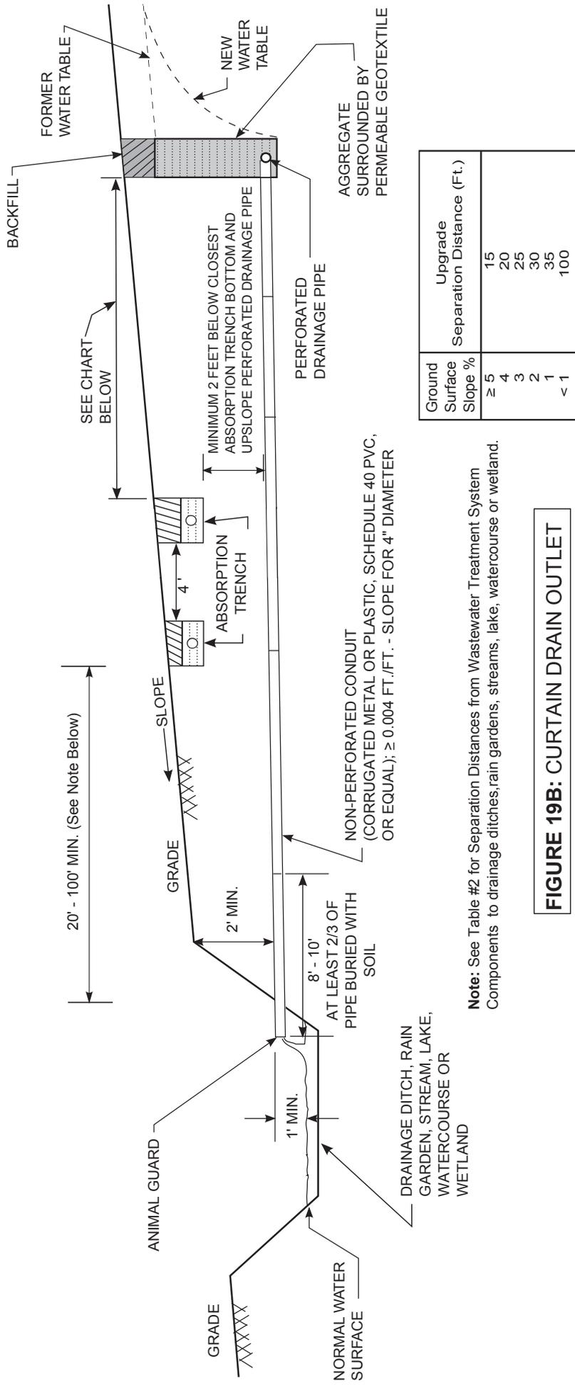
**Note:** See Table #2 for Separation Distances from Wastewater Treatment System Components to drainage ditches, rain gardens, streams, lake, watercourse or wetland.
