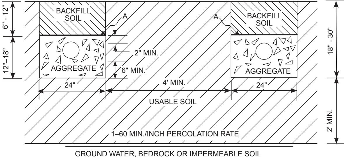
A = PERMEABLE GEOTEXTILE, UNTREATED BUILDING PAPER, OR 4" OF HAY OR STRAW.
