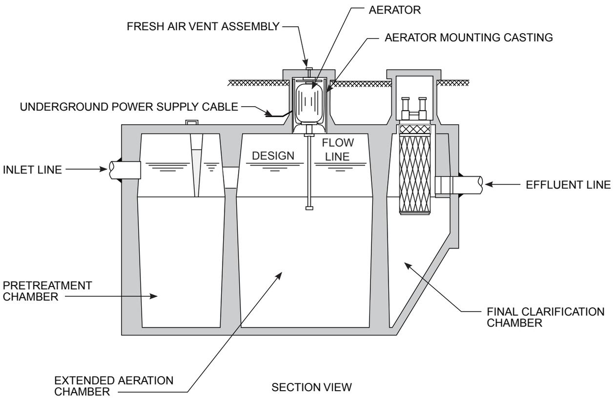
**FIGURE 8: EXAMPLE ENHANCED TREATMENT UNIT (ETU): SUSPENDED GROWTH (AERATED)**
