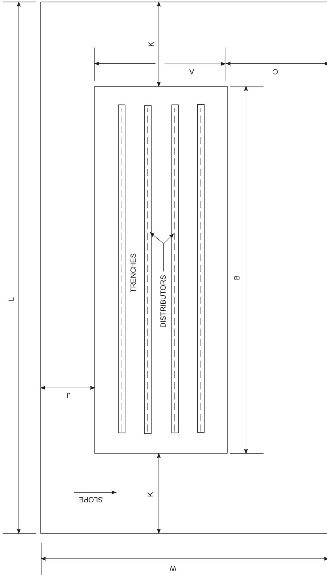
**FIGURE 30A: TYPICAL MOUND DIMENSIONS - TOP VIEW - ABSORPTION TRENCHES**
